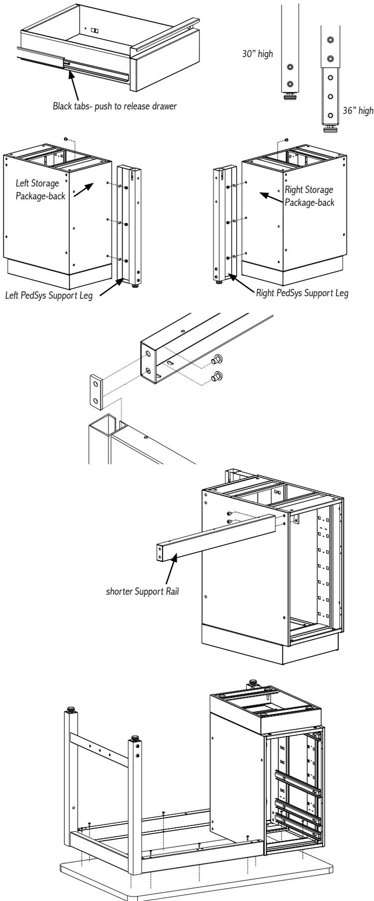
1. Remove drawers and/or pull-out shelves from the Storage Package by pushing up or down (depending on side) on the black tabs on both sides of the drawer slide and pull forward. Set aside.
