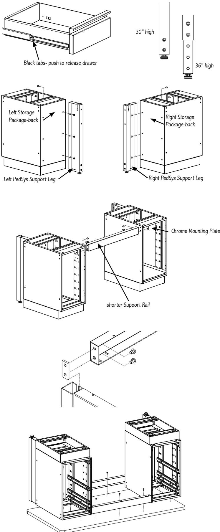
1. Remove drawers and/or pull-out shelves from the Storage Package by pushing up or down on the black tabs (depending on side) on both sides of the drawer slide and pull forward. Set aside.
